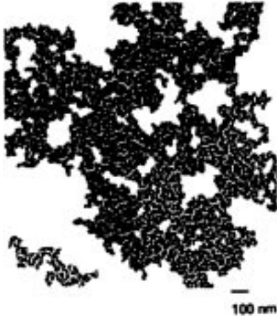
Fig. 5. Gold film evaporated on amorphous \text{Si}_3\text{N}_4 (after [6]).
